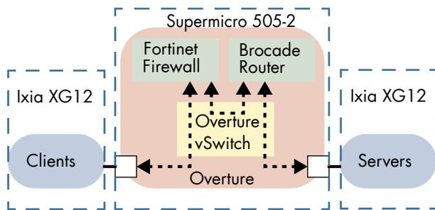
**Figure 1: Physical & logical EANTC test setup**
