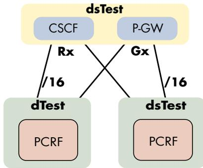
**Figure 1: Developing Solutions PCRF Test Setup**
