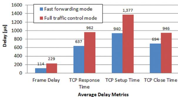
**Figure 5: Delay Measurement with & without Traffic Control Function**
