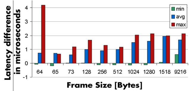
**Figure 3: Latency Differences Results Between Port Controllers**
