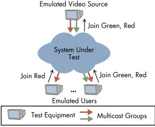
**Basic Multicast Black Box Test Setup**
