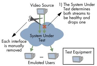
If the system under test does in fact make use of both video flows to truly provide lossless video, both 0 frame loss and no changes in video quality will be observed throughout the test. To note, this procedure assumes that each of the two identical video flows will enter the network on a separate interface. If this is not the case, information relating to how each flow traverses the network must be known in order to remove a link which only affects a single flow.
