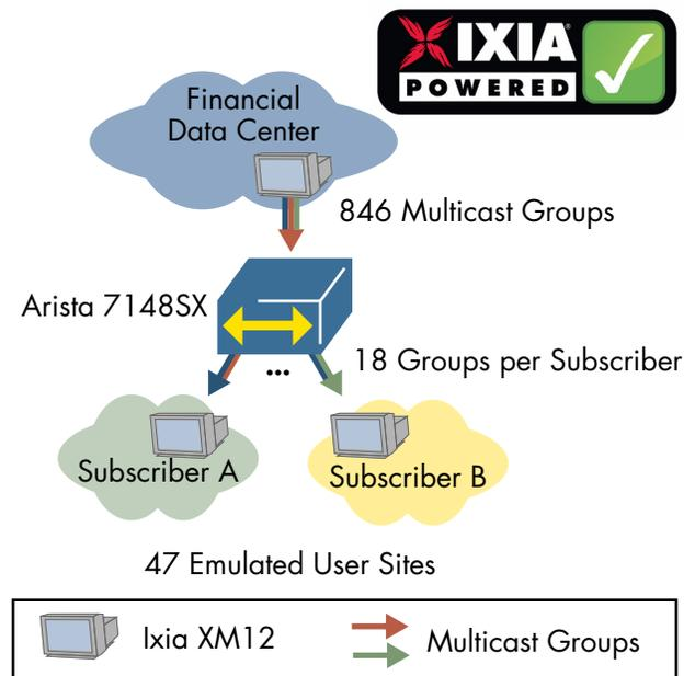
**Figure 2: Distributed Multicast Throughput and Latency Test Setup**
