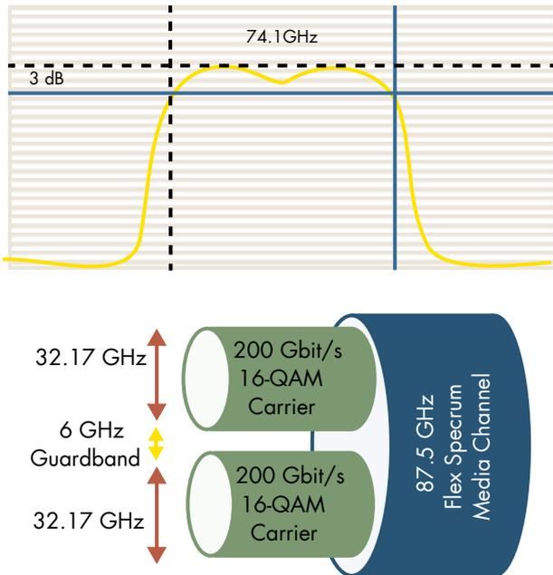
**Figure 2: Flex Spectrum Configuration and Optical Spectrum Analysis**
