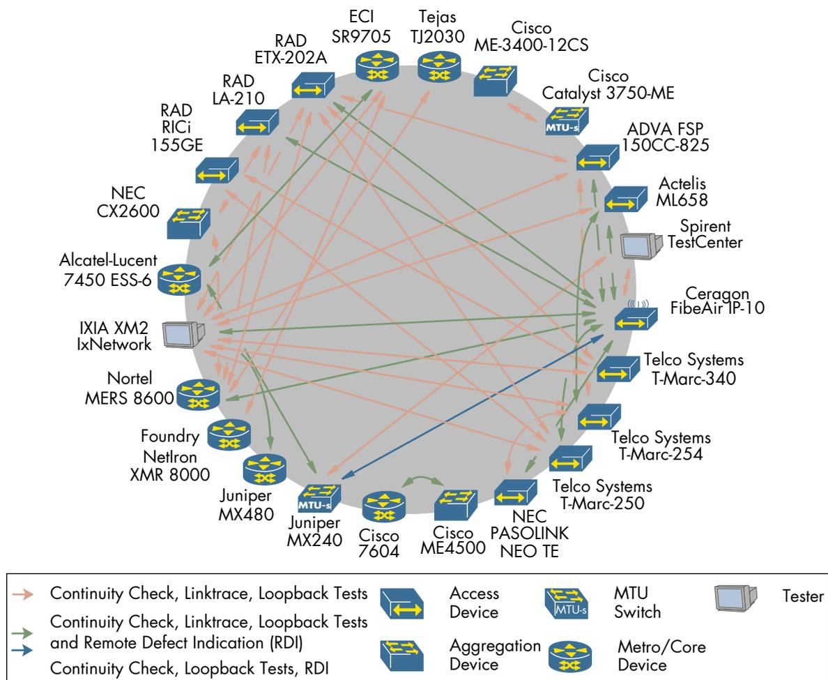
Figure 9: Service OAM Test Results
