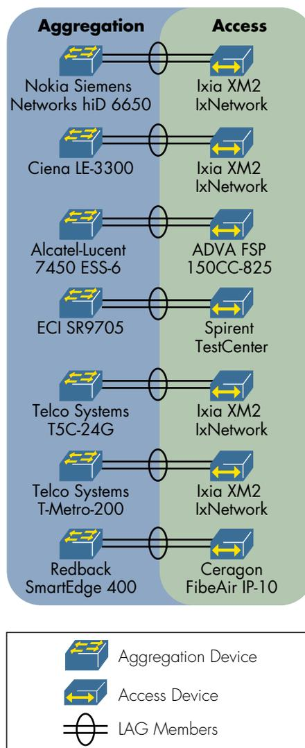
**Figure 11: LACP test pairs**
