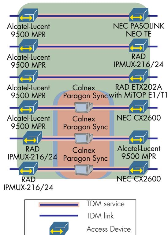
Figure 5: CES tests back-to-back
