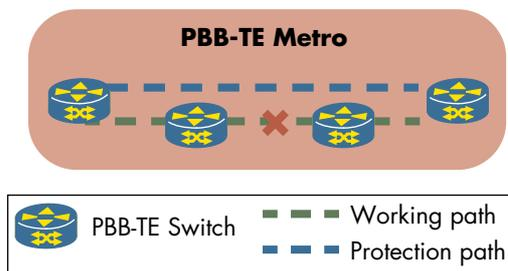
**Figure 4: PBB-TE Protection Setup**
