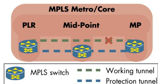
Figure 3: MPLS Fast Reroute Test Setup
