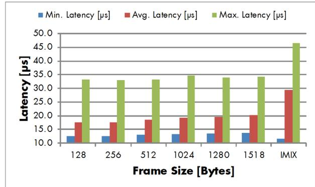
**Figure 12: IPv4 Forwarding Delay**
