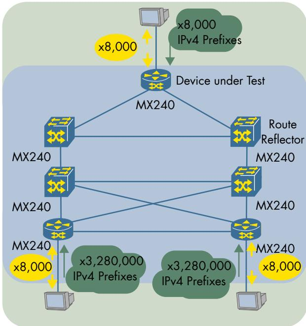
**Figure 4: L3VPN Scalability VRF Instances Test Setup**
