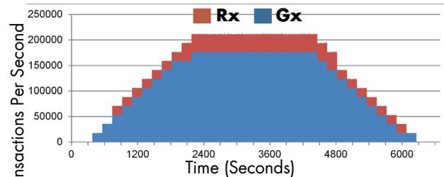
**Figure 3: Transactions Per Second Combined Gx and Rx Interfaces**
